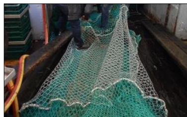
First panel in T90 on the sorting yard (ship THE ECUME DES JOURS) © Cobrenord
